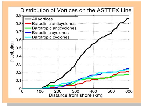
Vortices detected by the pressure sensor equipped inverted echo sounders (PIES) on the ASTTEX line were fairly evenly distributed among baroclinic cyclones and anticyclones, and barotropic cyclones and anticyclones.
