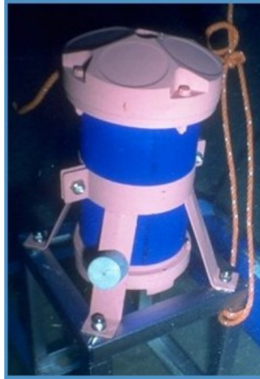
Figure 59. Antifouling Paint Applied to a WorkHorse Sentinel
