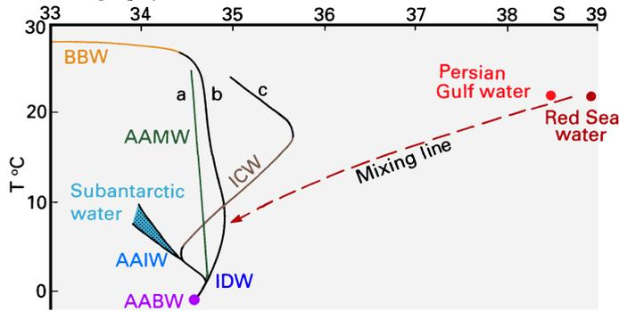
Fig. 12.5. T-S diagram showing the source water masses for the Indian Ocean and their effect on the temperature - salinity structure in different regions. Curve *a* is representative for the region between Australia and Indonesia (120°E), curve *b* for the Bay of Bengal (88°E) to 10°S, curve *c* for the subtropics south of 10°S. Intrusions of Red Sea and Persian Gulf Water can produce departures from the T-S curves near the isopycnal surface  $\sigma_t = 27.2$  (the "mixing line").
