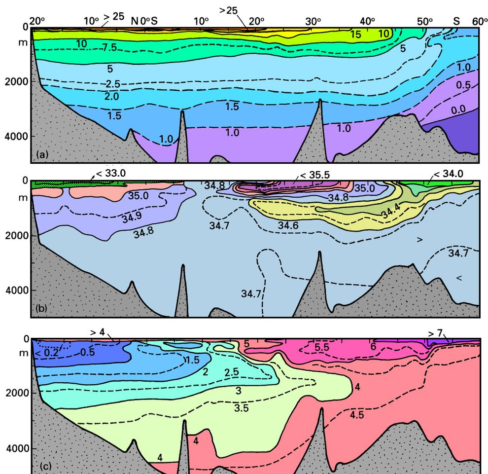
Fig. 12.4. A section across the Indian Ocean along approximately 95°E. (a) Potential temperature (°C), (b) salinity, (c) oxygen (ml/l). From Wyrтки (1971). See Fig. 12.1 for location.
