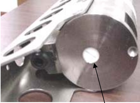
Pressure sensor port plug
