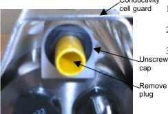
The SBE 16*plus* has an anti-foul cup and cap on each end of the conductivity cell. A new SBE 16*plus* is shipped with an anti-foul cylinder and a protective plug pre-installed in each cup.
