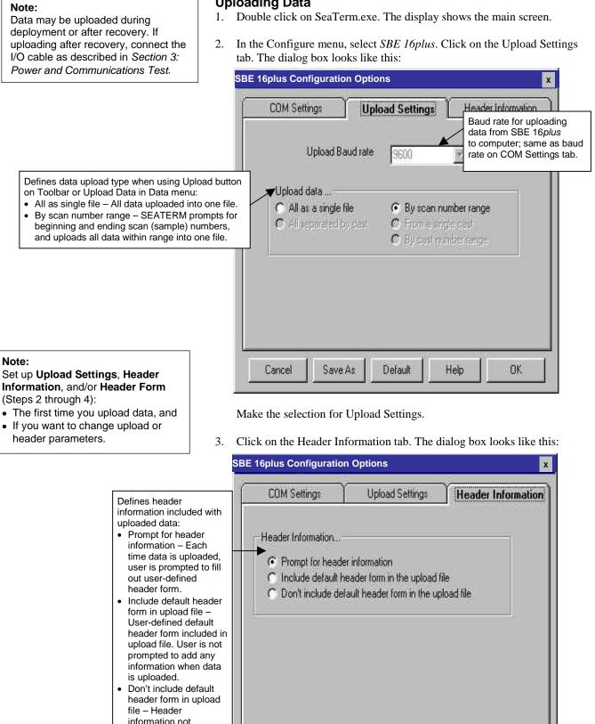
Select the desired header information option. Click OK to overwrite an existing COM/Upload/Header Settings file, or click Save As to save the settings as a new filename.
