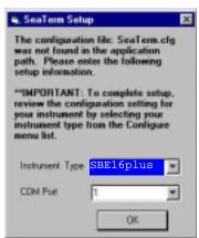
Select the instrument type (SBE 16plus) and the computer COM port for communication with the SBE 16plus. Click OK.
